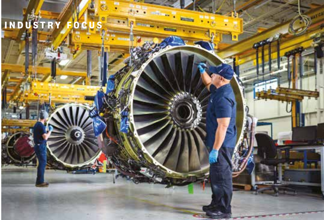
1. A CFM56-7B fan inspection is performed at StandardAero facilities 2. STS Aviation Group provides aircraft maintenance, engineering, recruiting and component services to the global aviation industry – with about 30-40 per cent of its revenue coming from international origins
