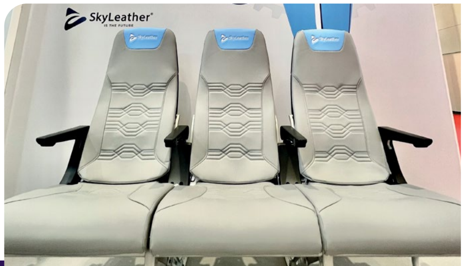
Nose to tail: AJW Technique Interiors’s replacement seat covers use SkyLeather synthetic leather.
