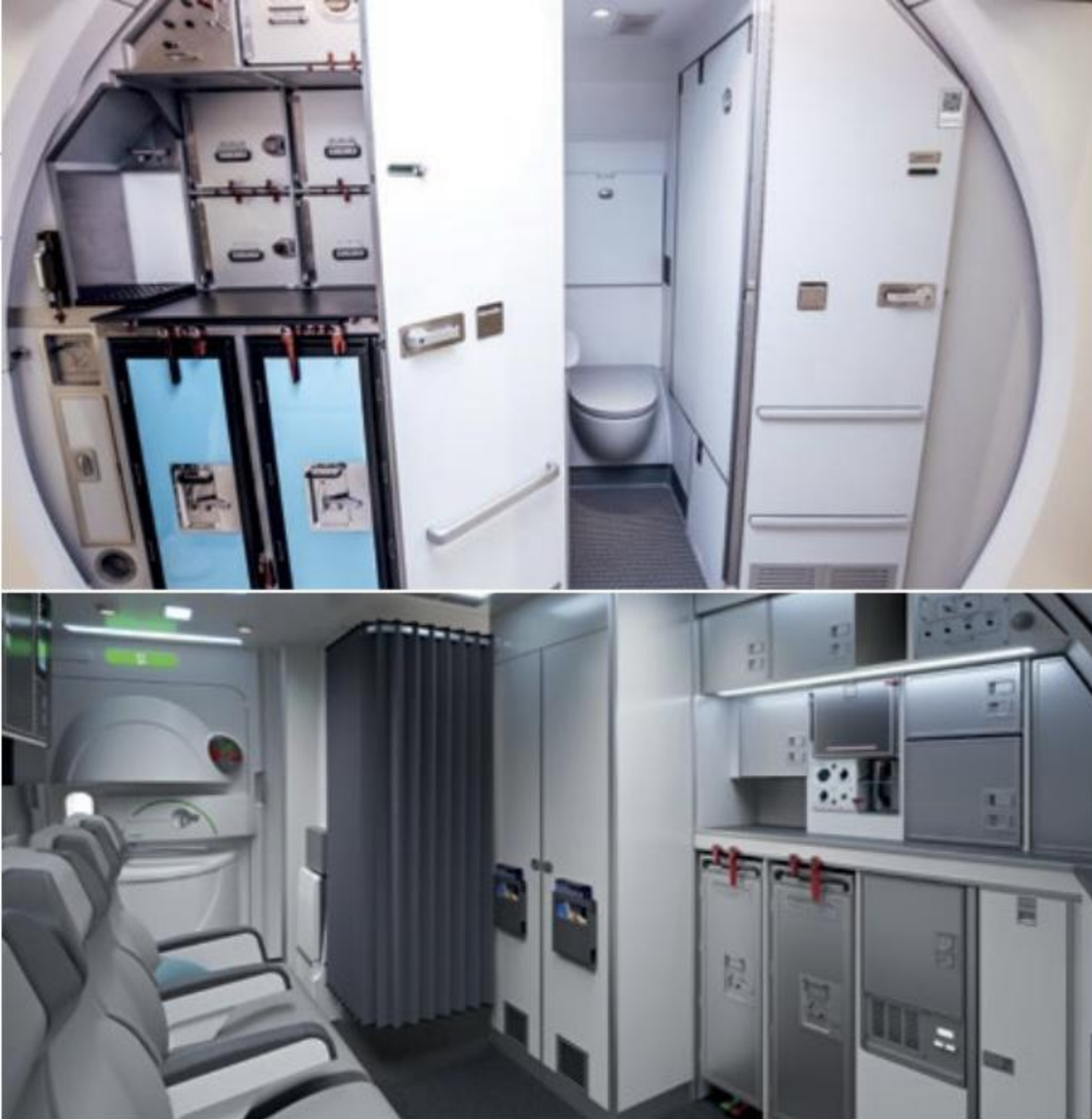
Diehl's AirPax module comprises one galley and two lavatories and weighs 60 kg less than standard solutions.
